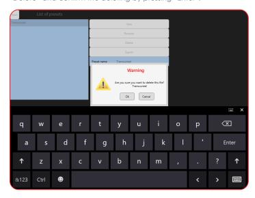
If the preset selected for delete is loaded and in use, the device will delete it and a default preset will be loaded instead.
