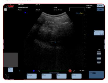
Place the first grey caliper with the touchpad in the desired place to start to measure the distance D1. Press "Set". The second caliper is now displayed.
