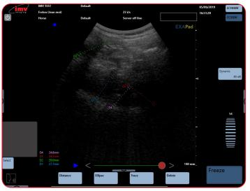
The control "Toggle" enables you to go from one caliper to the next in order to adjust the measurement before validating.
