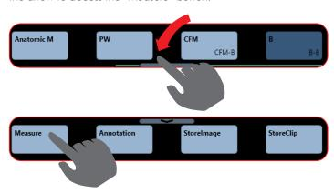
Activate/deactivate measurement controls by pressing "Measure" after freezing the image.
