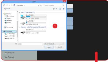
Select Driver: enables the driver selection for the installation of a new printer. Before installing a new printer, press "Select driver" and a new window opens. Search the hard disk or an external support for the driver of the printer to be installed and follow the installation procedure.
