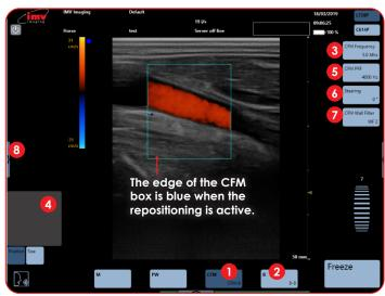
The colour scale which is also the PRF scale is graduated in two parts in order to distinguish the two directions of the flows: towards and away from the probe. Slow flows are depicted in dark red or dark blue; high speeds are passing from blue to white or from red to yellow (depending on the direction).
