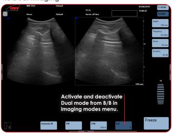
The image on the right of the screen is live. Touch the left image in order to freeze the first image and activate the second.
