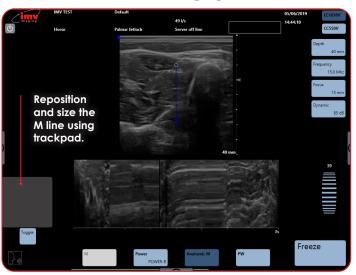
Place the start of the Anatomic M line with the trackpad, then press Toggle in order to position the arrow that symbolises the end of the Anatomic M line specter.
