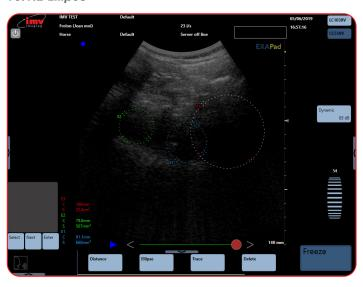
Place the first grey caliper (E1) with the trackpad to start to measure the ellipse. Press "Set". With the trackpad, draw the measurement and press "Enter" to validate.
