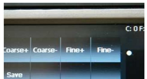
11. then do the same thing with Fine function, put it first at '0' and then adjust the image with Fine + and Fine -.(there are values from 0 to 15).
